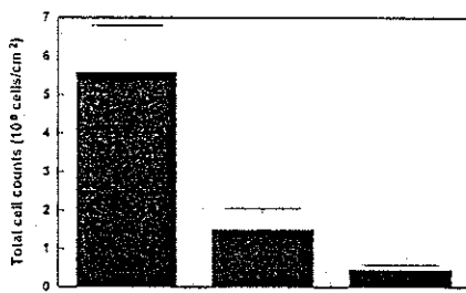
Fig. 3. Microscopic counts of acridine orange-stained biofilm cells after 96 h exposure to chlorine.
